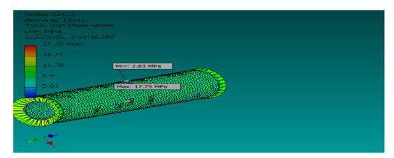
Figure 4.6: Simulation of the Effect of Pressure at 6.2052 MPa(900 psi) on a 11 inch Pipe
