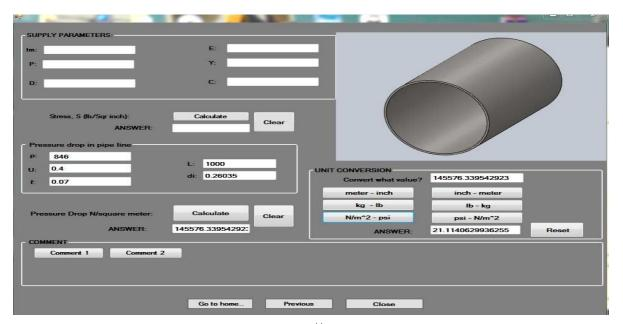
Figure 4.7: Result Obtained from C<sup>++</sup> Programme Showing the Stress That was Induced in the Pipe during Failure
