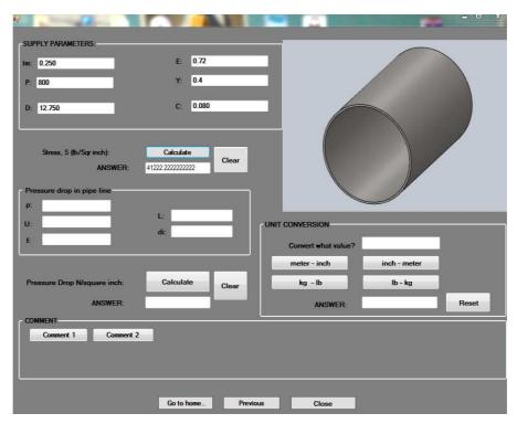
Figure 4.1: C<sup>++</sup> Programme Interface Showing the Calculation of Stress Exacted on the Pipe at 800 Psi
