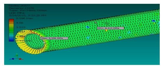
Figure 4.3: Simulation of the Effect of Pressure at 5.5158MPa (800 psi) on a 12 Inch Pipe
